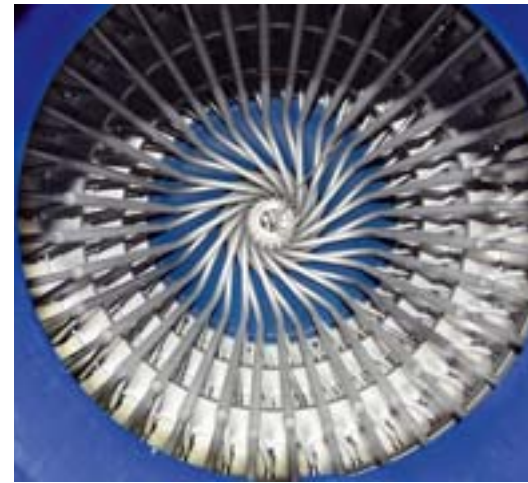
Filtrate drainage pipes to the control head inside the filter drum of a rotary pressure filter
