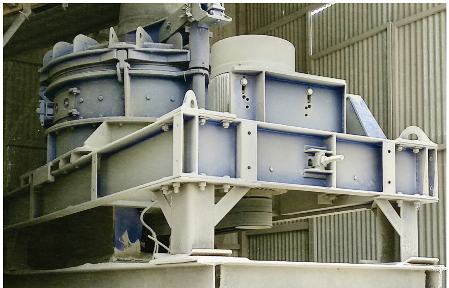
Kasprs Build Mate's RPM 1513 rotor impact mill from BHS-Sonthofen
