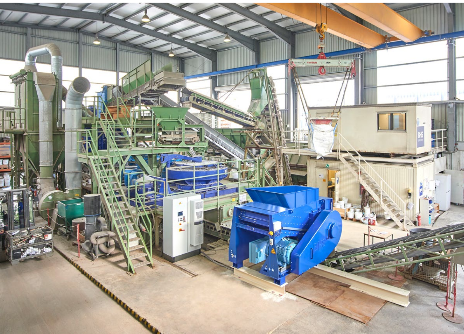
Universal Shredder NGU 0513 for testing at the BHS technical center in Sonthofen.
